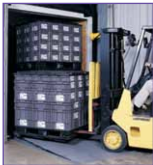
The modular design cubes the AIAG standard 48" x 45" pallet for maximum space usage.
